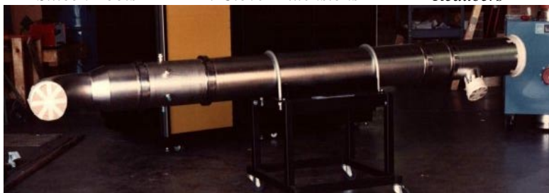
Diesel Dilution Tunnel
